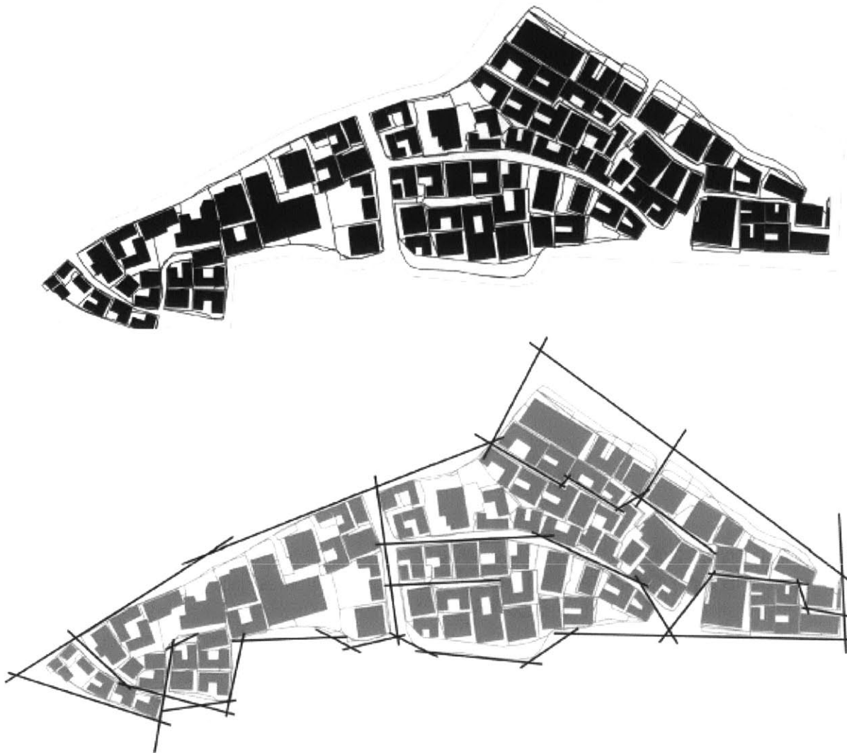
Figure 0-2. The spatial structure of open space and its axial representation (Hillier, spacesyntax.com)
