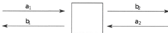
Figure 2-6: Incident and reflected waves in an electrical system
