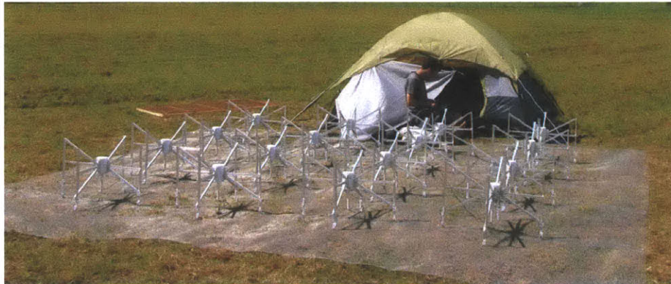
Figure 2-1: Array of MWA antennas in Green Bank, WV
