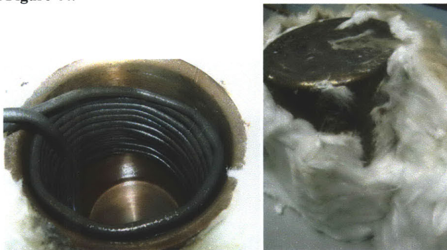
Figure 45: On the left, darkened stainless steel vessel and coiled copper tube heat exchanger after a 3-4 hour single run. On the right, insulation degradation close to the stainless steel container. The blackened copper layer can flake off thus releasing particulates into the molten salt.
