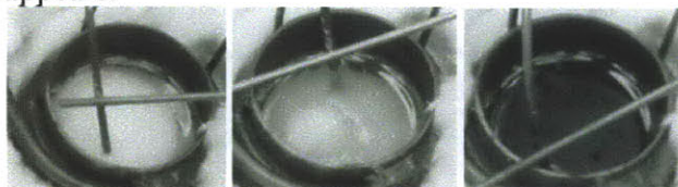
Figure 24: Series of images showing the melting process of the salt through out time. The image on the left is at the onset of melting. The center image shows the progression of melting from the sides and the sinking of the solid salt. The image on the right shows the fully melted salt bath.
