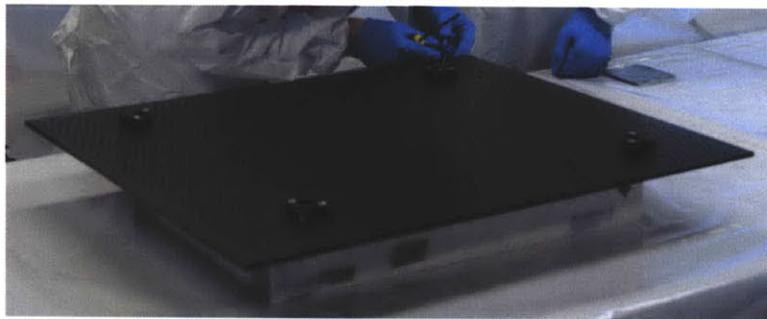
Figure 3-13: Kinematic couplings on document platen.
