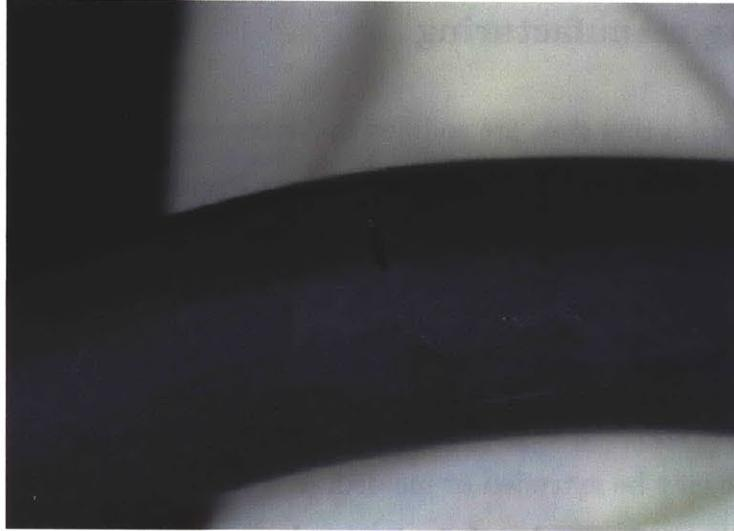
Figure 2-8: A defective splice in an extruded and centerless-ground o-ring.
