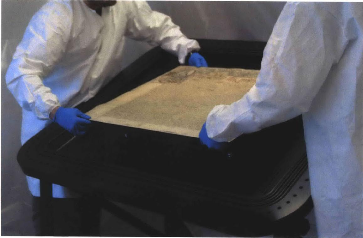
Figure A-14: The platen is installed in the tub.
