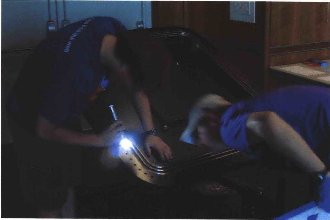
Figure 4-10: The encasement is inspected with low ambient light and a flashlight.
