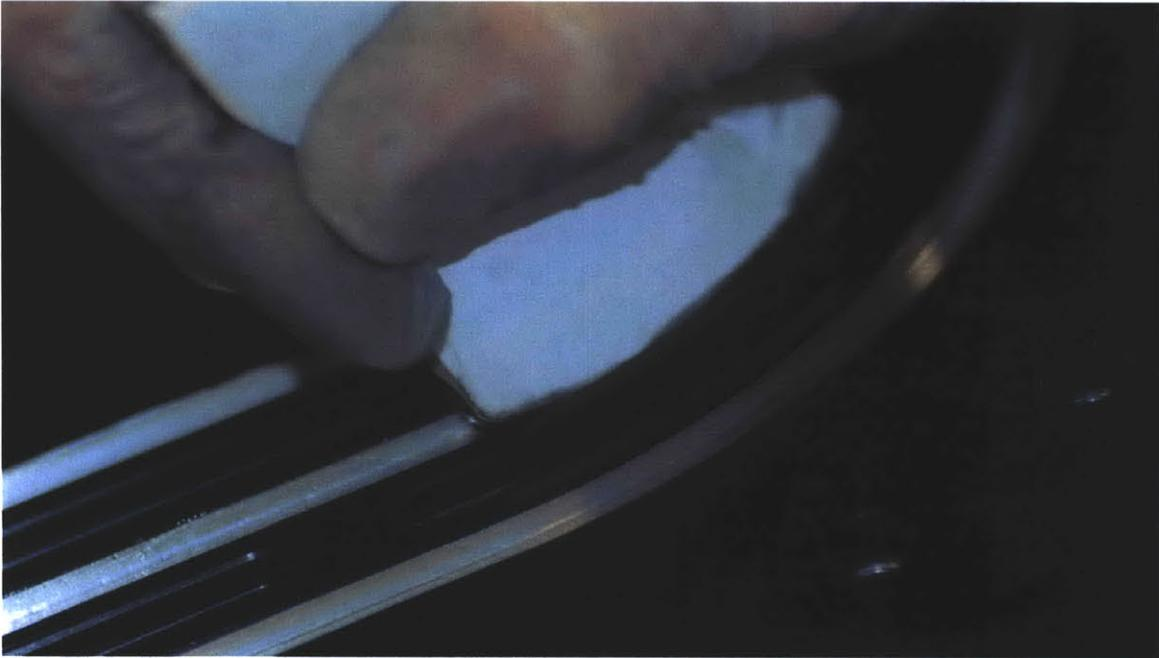
Figure 4-9: The o-ring groove is polished using foam poster board as a soft sanding block.
