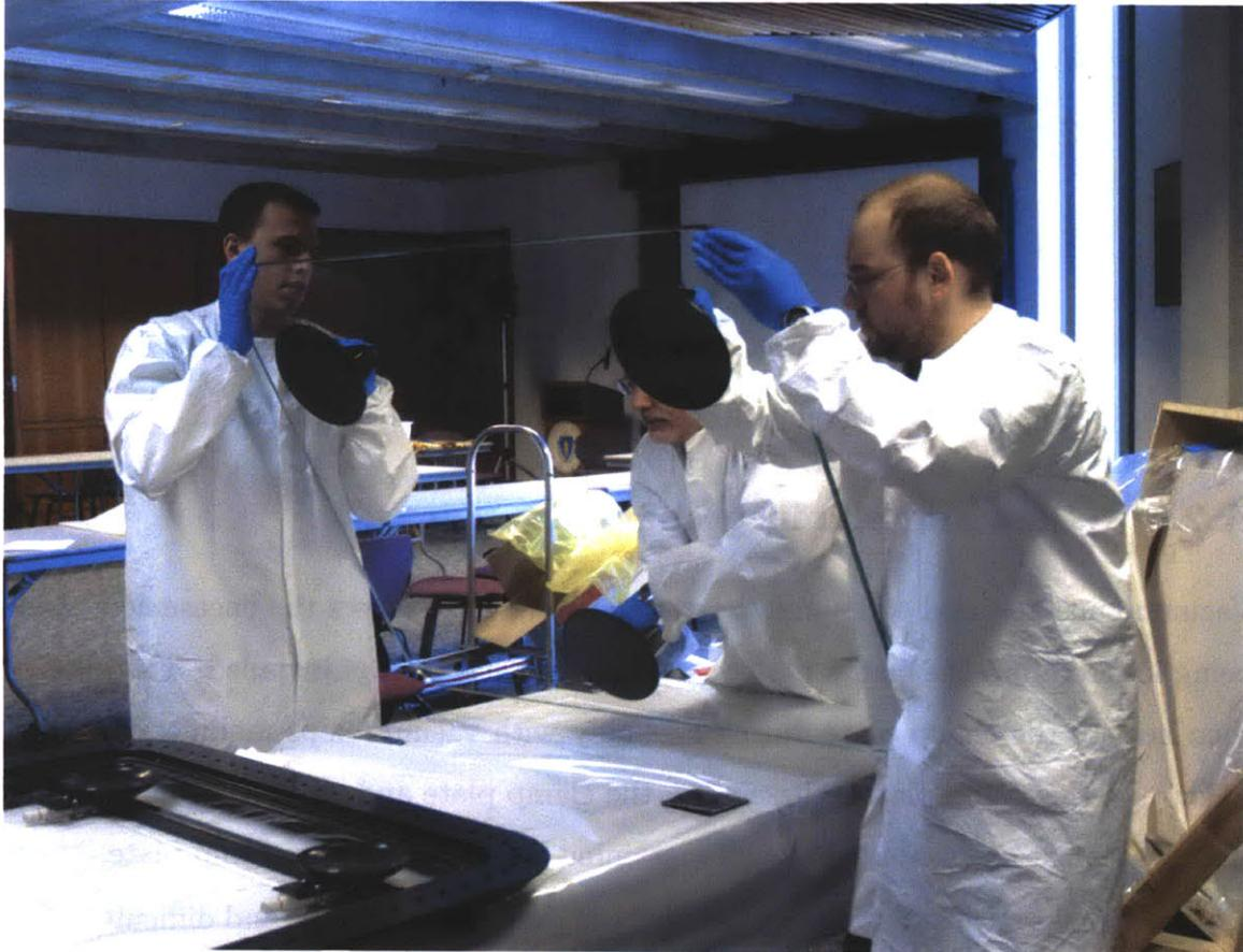
Figure A-10: The glass is lowered onto the clamp plate, after the o-rings are installed in the clamp plate.
