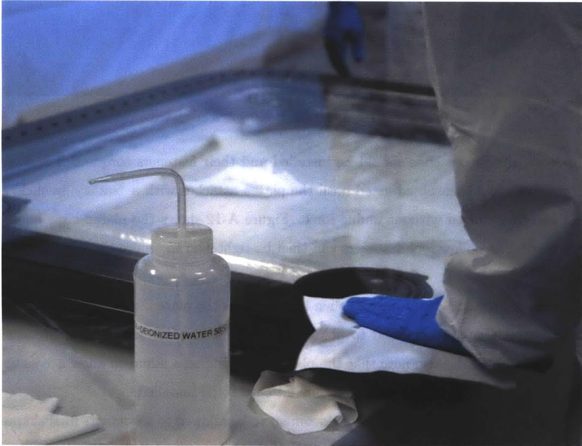
Figure A-11: Cleaning glass just before final assembly.
