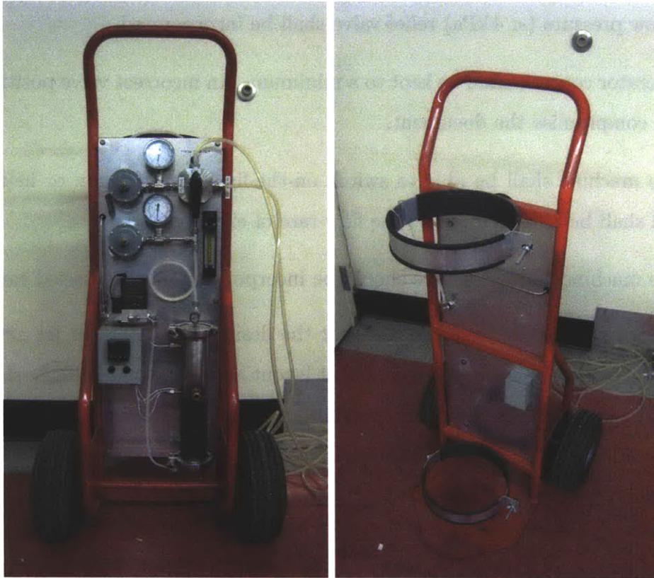
Figure 6-1: Completed Moisturematic (front and rear views)
