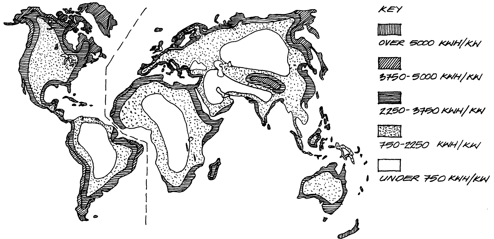
AVAILABILITY OF WIND ENERGY ON EARTH ANNUAL SPECIFIC OUTPUT OF WIND TURBINES RATED AT 25 MPH FIGURE 54 (FROM: WIND ENERGY CONVERSION SYSTEMS. NASA/NSF. 1973.)
