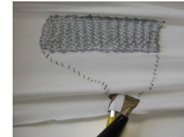
Figure 5. Stretch sensor made by knitting resistive yarn
