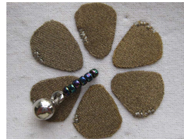
Figure 1: Tilt sensor made from conductive fabric, conductive thread and a metal bead
