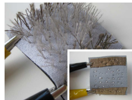
Figure 3: Stroke sensor made from neoprene and conductive thread
