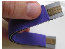
Figure 2: Neoprene bend sensor made from neoprene, conductive fabric, conductive thread, and Velostat
