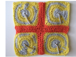
Figure 4. Series of crochet tilt potentiometers made from resistive and traditional yarn
