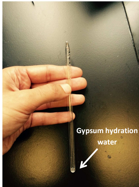
Figure S6. Gypsum hydration water recovered after a WASP run in a 6-mm break-seal tube.
