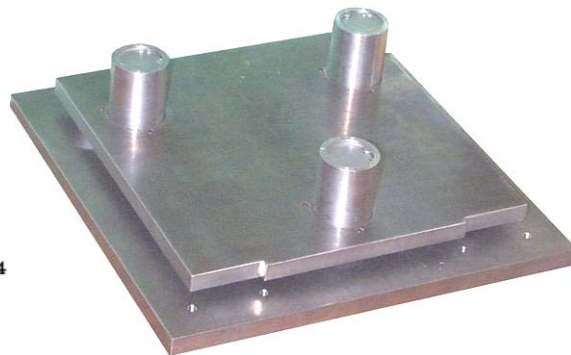
Figure 13 Kinematic coupling element constrained to move axially by a die-set bushing and spring washer stack. (Courtesy D. Braunstein)
