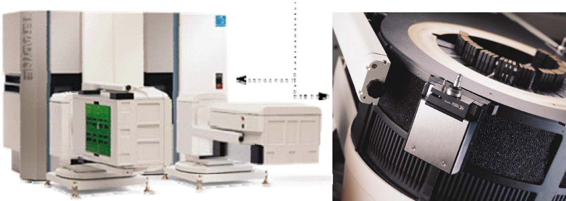
Figure 17b K-Docks used in precision alignment application for semiconductor test equipment. (Courtesy M. Chiu)
