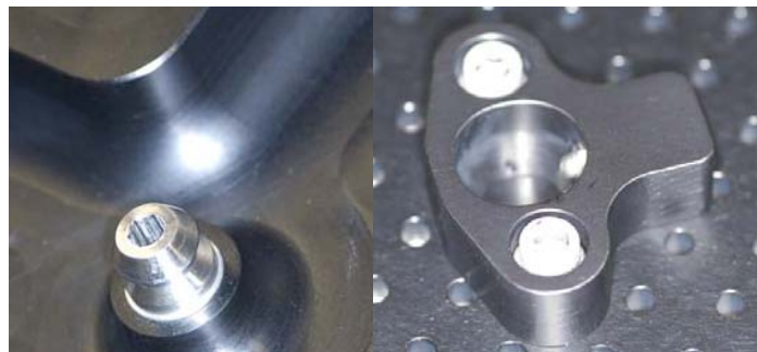
Figure 20b Split groove kinematic coupling elements made from a conical male (l) and mating grooves made from slots milled with a V cutter (r). A ball-spring plunger provides preload and manually removable snap-fit locking (Courtesy Massachusetts State Archives)
