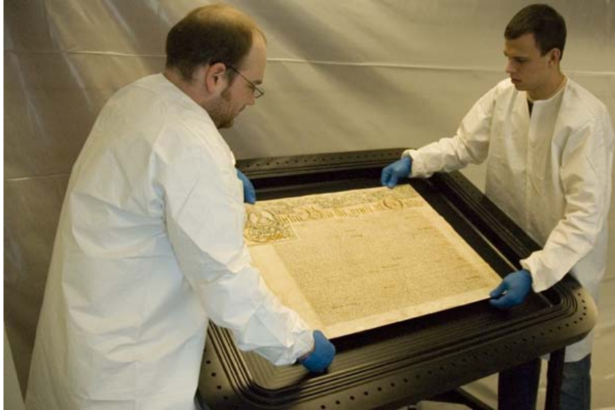
Figure 20c A platen holding a priceless document is held in position using split groove kinematic couplings in a special environmental display case (Courtesy Massachusetts State Archives)
