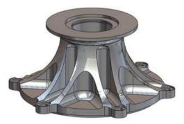
Figure 2.1 A fuel pump mount model designed by 3D CAD (free model download from http://3dprinterbaski.com/cadcam-sistemlerinin-genel-yapisi)
