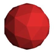
Figure 6.17 All pixels on the same polygon are given the same colour in Flat shading
