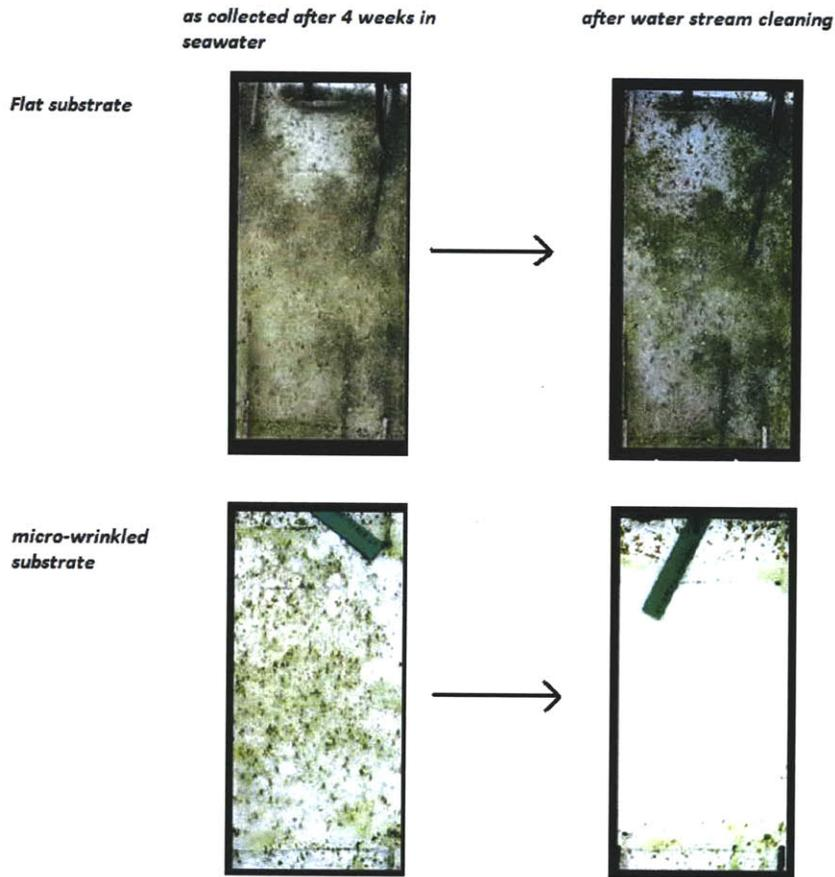
Figure 36: Comparison of flat PDMS (top figures) and unidirectional wrinkled PDMS (bottom figures) after 4 weeks exposure in a marine environment. Anti-adhesion performances are assessed by the differential color of the two samples as remove from the seawater. Removal properties are assessed by the differential color before and after rinsing the sample with a water stream (from (72) )
