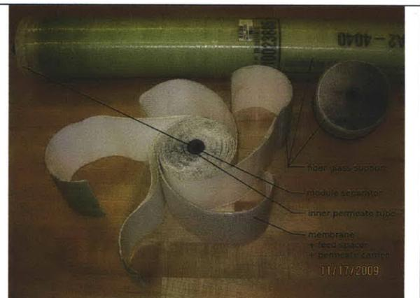
**Figure 9: Picture of the cross section of a Filmtech 8inch element.** Several sheets are wrapped around the permeate collector. The element is inserted into a fiberglass case (green), which is itself inserted into a pressure vessel.
