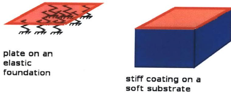
Figure 67: Two possible modelings for the problem: a/ plate laid on top of an elastic foundation b/hard coating (shell or 3D continuum modeling of the coating) on top of a substrate
