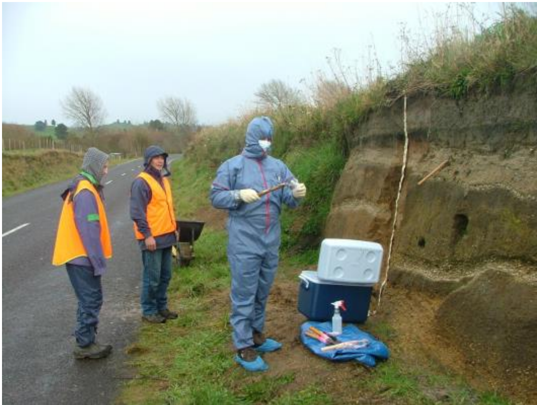
Fig. A2 Sampling for PalEnDNA in paleosols on tephras: (1) soil profile should be excised laterally to remove surface contamination, (2) tools for sampling must be sterile, and (3) protective gear, including gloves, disposable body suit and face mask are required to avoid any extraneous DNA from the sampler. Photo: D.J. Lowe.
