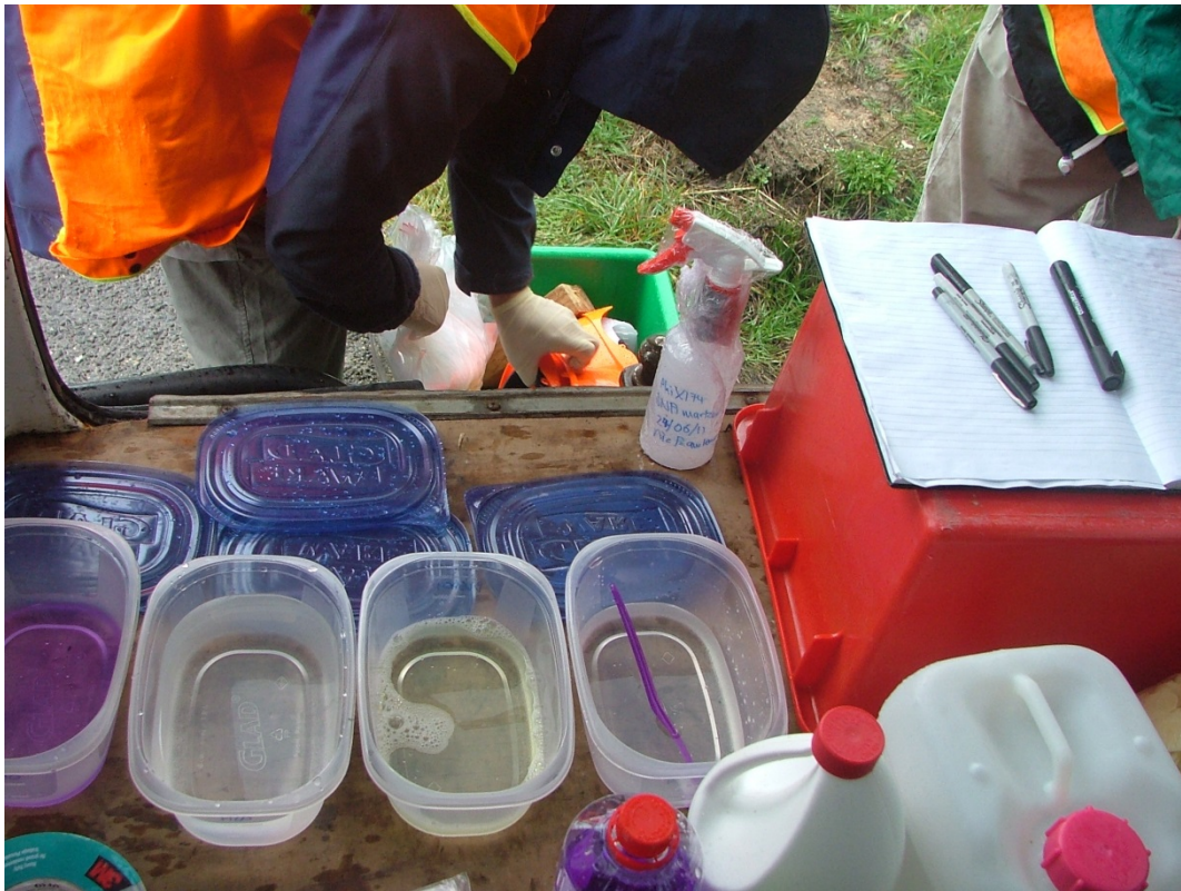
Fig. A4 An array of chemicals/solutions, including water, detergent, ethanol, and disinfectant, used to wash sampling tools to ensure they remained sterile for each use.
