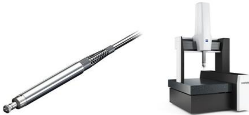
Figure 2. 2 Analog touch probe (left) [14], Bridge coordinate measuring machine(right)[15]
