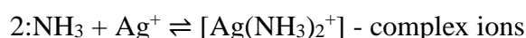
Figure 2.10: Complex formation between an electron pair donor (a base) and an electron pair acceptor (an acid) where NH_3 is the ammonia ion as the base, Ag^+ the Argentum ion, Ag(NH_3)_2^+ diamminesilver(1) (from Barcza & Buvári, 2003, p. 823)
