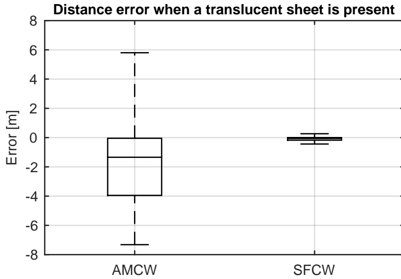
Figure 5.10: Box plot of the distance measurement error of pixels behind a translucent sheet for both the AMCW and SFCW measurements from figure 5.7 (d) and (h). The central mark is the median, the edges of the box are the 25th and 75th percentiles, the whiskers extend to the most extreme datapoints and the outliers have been removed.
