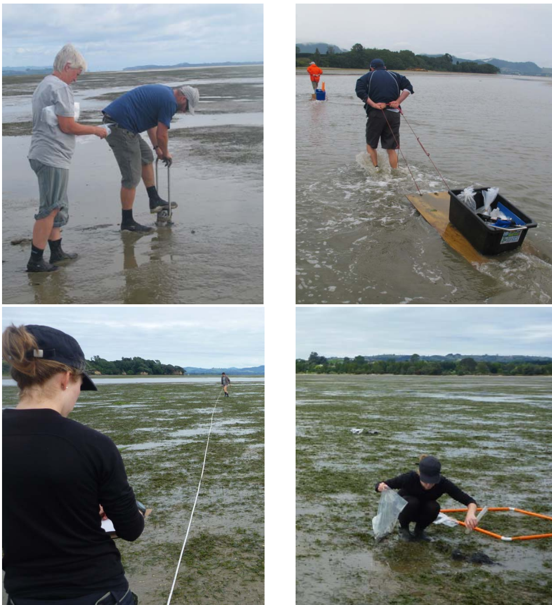
Figure 2. Photographs of sampling procedure. Clockwise from top left: taking infauna core; transporting samples; sampling for surface sediments with quadrat for photographs nearby; measuring out grid.
