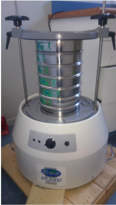
Figure 26. Endecott's EFL2000 sieve shaker used for grain size analysis.
