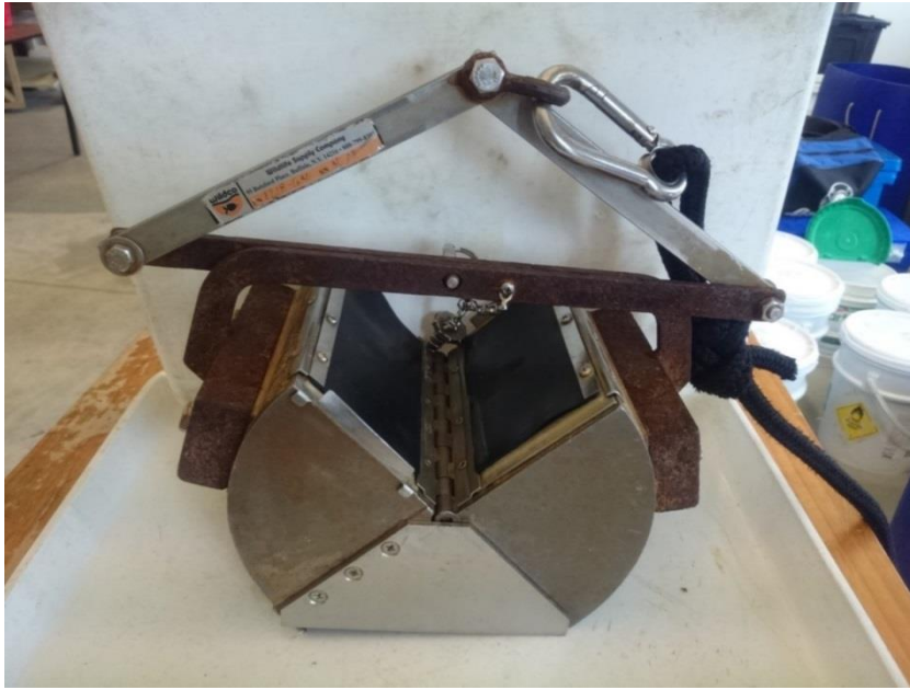
Figure 25. Ponar grab used for sediment sampling.
