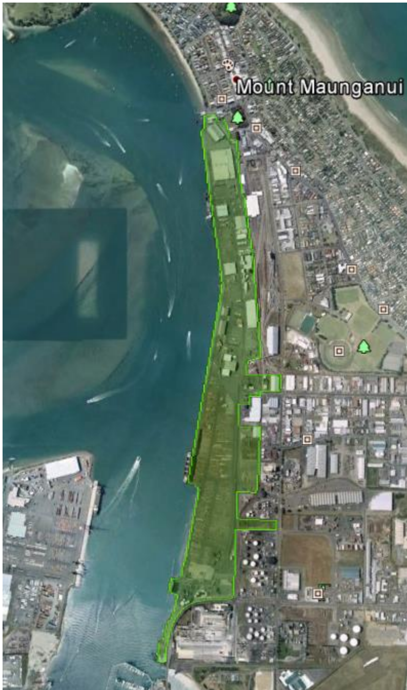
Figure 3.8: Port area, to calculate runoff producing area with Google Earth Pro polygons. Area approximated from Figure 2.2.
