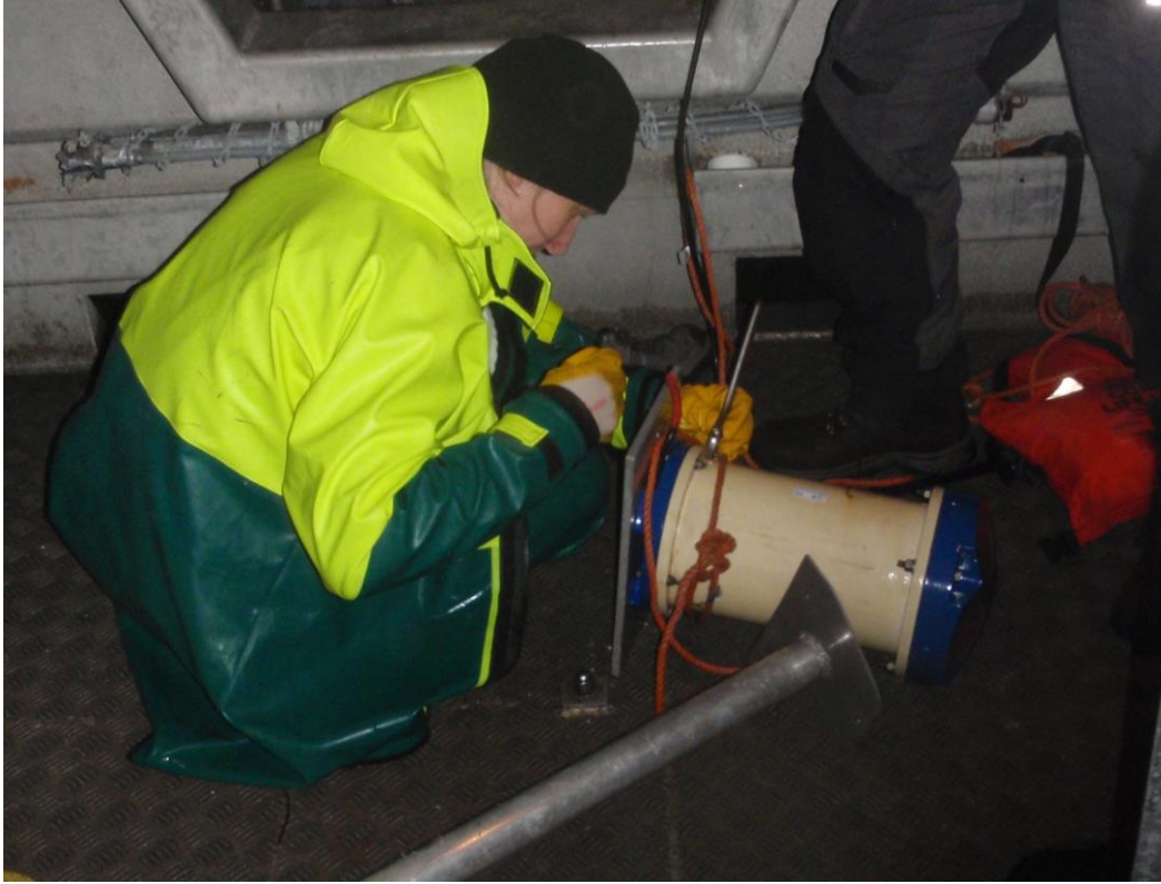
Figure 4.11: Julia Mullarney is disassembling the RDI ADCP workhorse after a day in the field (photo credit: Nadine Brunswiler).
