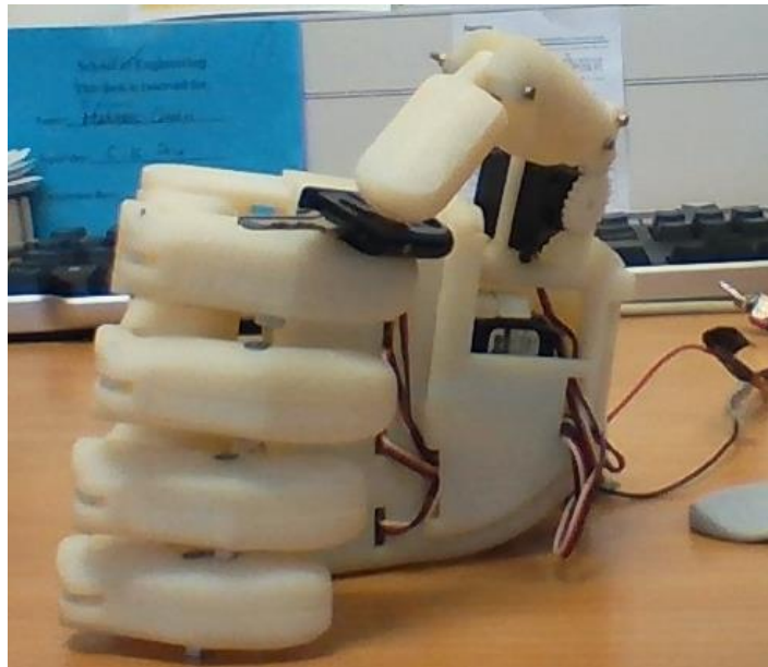
Figure 4.14: Execution of key grip by designed hand.
