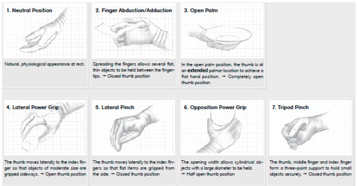
Figure A 22: Grips and grasps that can be accomplished by the Michelangelo hand. [49]
