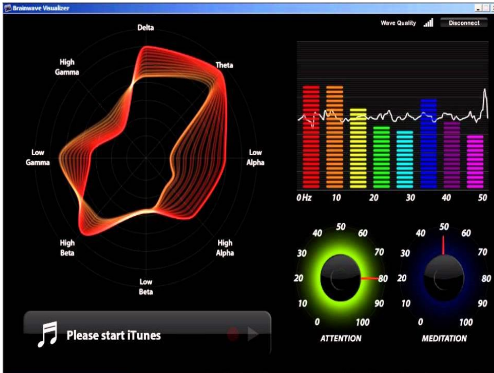
Figure 4.1: Screenshot of the Mindwave mobile core program showing an elevated reading of attention.
