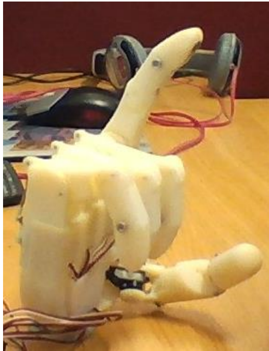
Figure 4.11: Execution of index point by designed hand.
