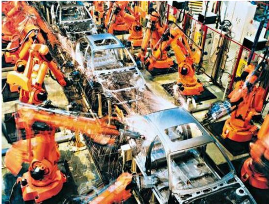
Figure 2.11: An assembly line using assembly robots to complete the welding of car chassis. [31].
