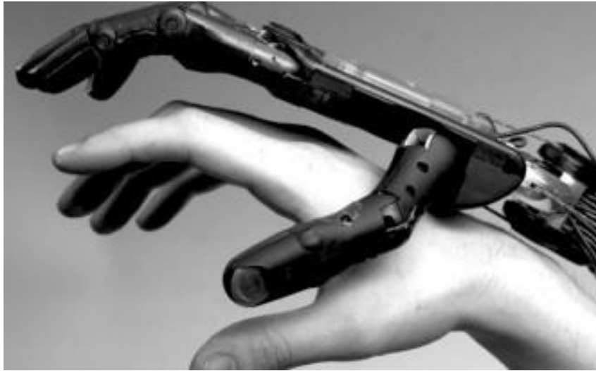
Figure A 14: The shadow hand in comparison to a human hand. [74]
