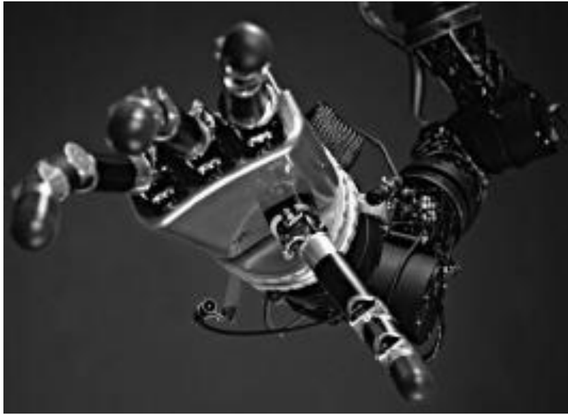
Figure A 20: DLR 1 hand. The model preceding the DLR 2 hand. [43]
