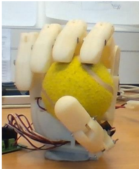
Figure 4.10: Execution of ball grip by designed hand.
