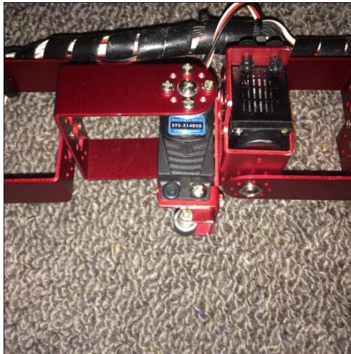
(b) U-shape brackets linking the joints
