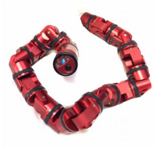
Figure 2.2 SEA snake robot which enables the torque sensing
