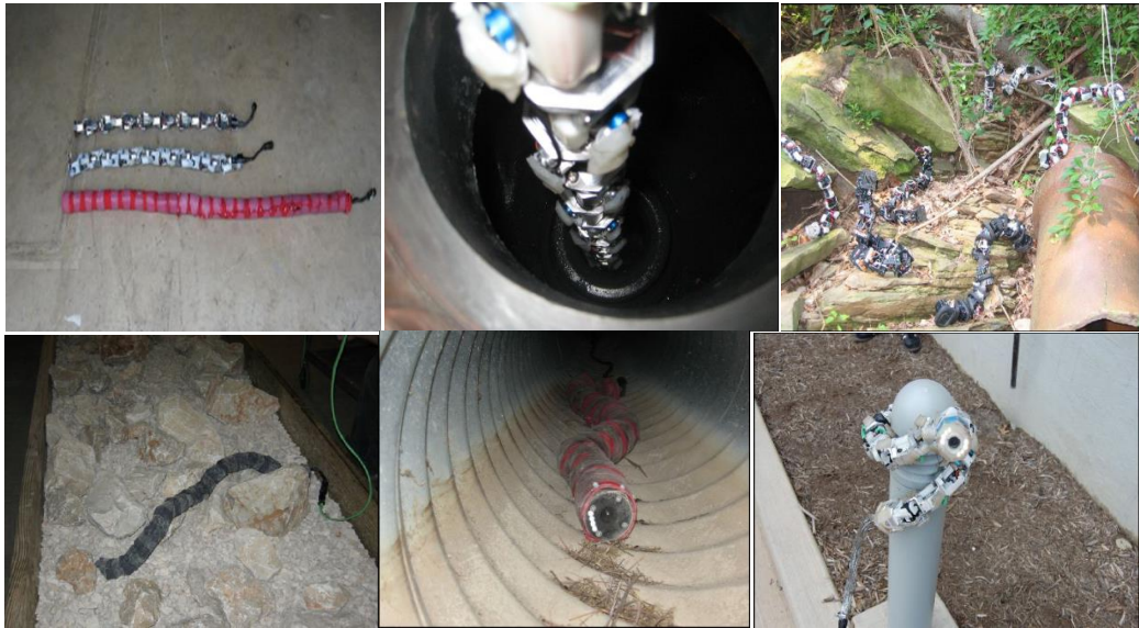
Figure 2.7 CMU snake robots with different covers in different terrain
