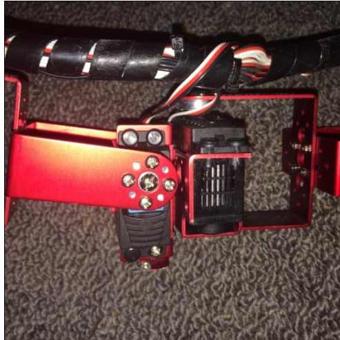
(a) Two servo brackets with two servo motors
