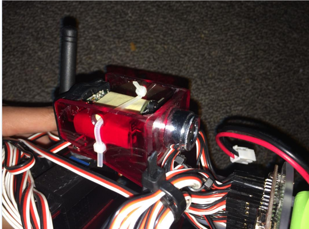
Figure 5.4 The wireless camera
