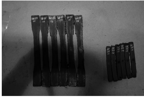
Figure 36 Specimen for injection moulded material
