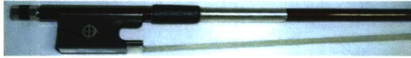
Figure 3.13: The CodaBow Colours bow stick is finished with a special paint that is highly reflective and causes it to appear to change color in the presence of different light sources. This cosmetic feature renders it unsuitable for strain gauge installation.
