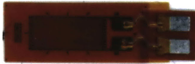
Figure 3.7: This uniaxial strain gauge (EK-06-250BF-10C) has a nominal resistance of 1000\Omega and is designed to measure strain in the direction of its grid lines. Its grid is composed of modified Karma, or K-alloy (nickel-chromium), an alloy characterized by good stability and fatigue life and a relatively flat thermal output curve. (The gauge grid is 6.35mm long and 3.18mm wide, and the dimensions of the entire object are 13.2mm long and 5.6mm wide.)
