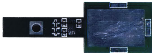
Figure 3.4: The printed circuit board antenna was designed to be secured to a threaded rod mounted to the tailpiece of a violin so that it was suspended just behind the bridge, with its large electrode facing toward the scroll of the instrument. The electronics on this board consisted only of the small circuit used to amplify the signal from the electrode (which is 0.859in long and 0.575in wide), and three LEDs so as to provide the option of indicating power and the varying strengths of the two signals transmitted from the Hyperbow .
