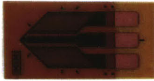
Figure 3.8: This is a two-element pattern (CEA-13-062UV-350) in which there are two gauges oriented such that they may measure shear, or torque strains. The devices are composed of A-alloy, or constantan, a nickel-copper alloy, the oldest and most common of strain gauge alloys. (The dimensions of the gauge grids are 1.57mm long and 1.60 wide each, and the dimensions of the entire object are 10.7mm long and 5.8mm wide.)
