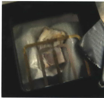
Figure 5-6 – For measurements at the medial tibia bone surface, the tibia was sectioned and approximated and attached to the membrane surface. The ESW devices were positioned on the opposite side of the membrane in a water bath.
