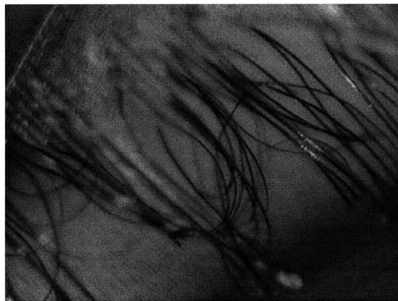
Figure 4-14: \text{XeF}_2 can attack the IDT electrodes especially by undercutting the adhesion layer (Ti).
