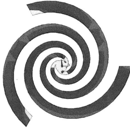
Figure 3-6: Strain distribution in geometry-optimized tri-spiral design with a heavy central proof mass.
