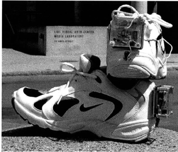
Figure 2-9: Parasitic power shoes project at MIT Media Lab (from [9])
