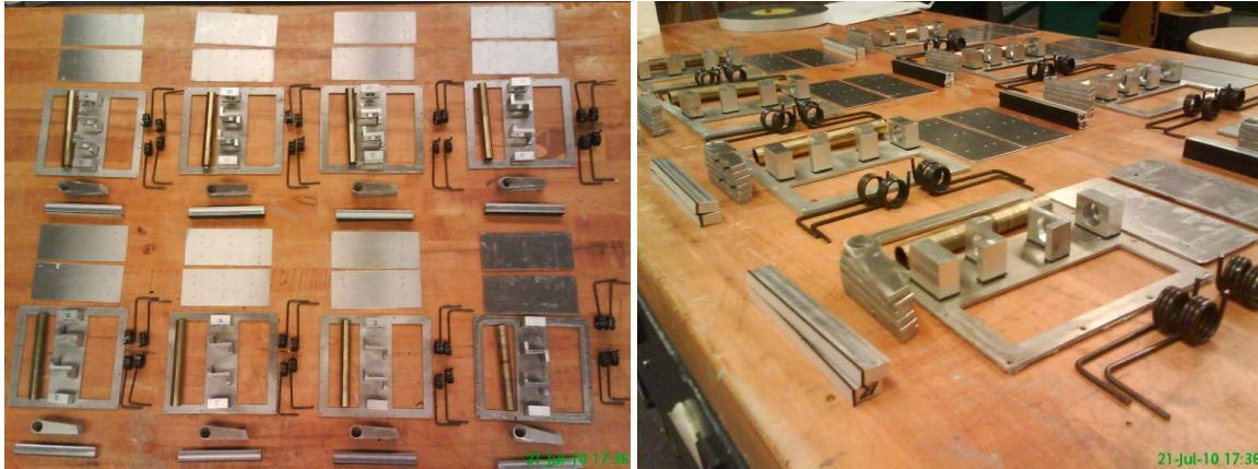
Figure 6-22: Manufactured Generation 3.1 Pressure Relief Valve Components
