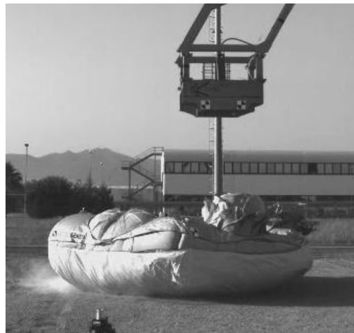
Figure 2-21: Drop testing of a prototype of the ExoMars airbag system [48]
