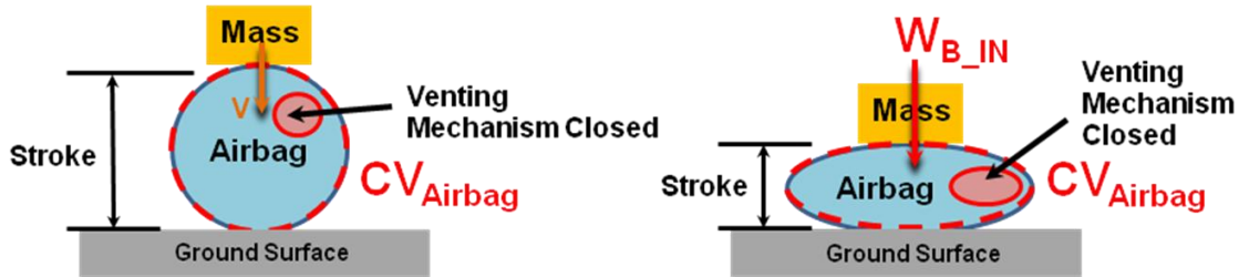
Figure 3-2: System State Transition between Initial Contact with the Ground and Maximum Airbag Compression
