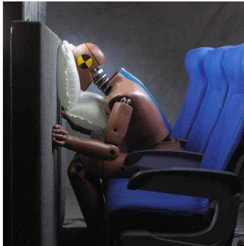
Figure 2-8: Amsafe Commercial Aviation Seatbelt Airbag [21]
