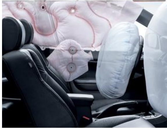
Figure 2-10: Airbag system in a 2007 Model Honda Accord automobile consisting of steering wheel mounted, side, and side curtain airbags [23]
