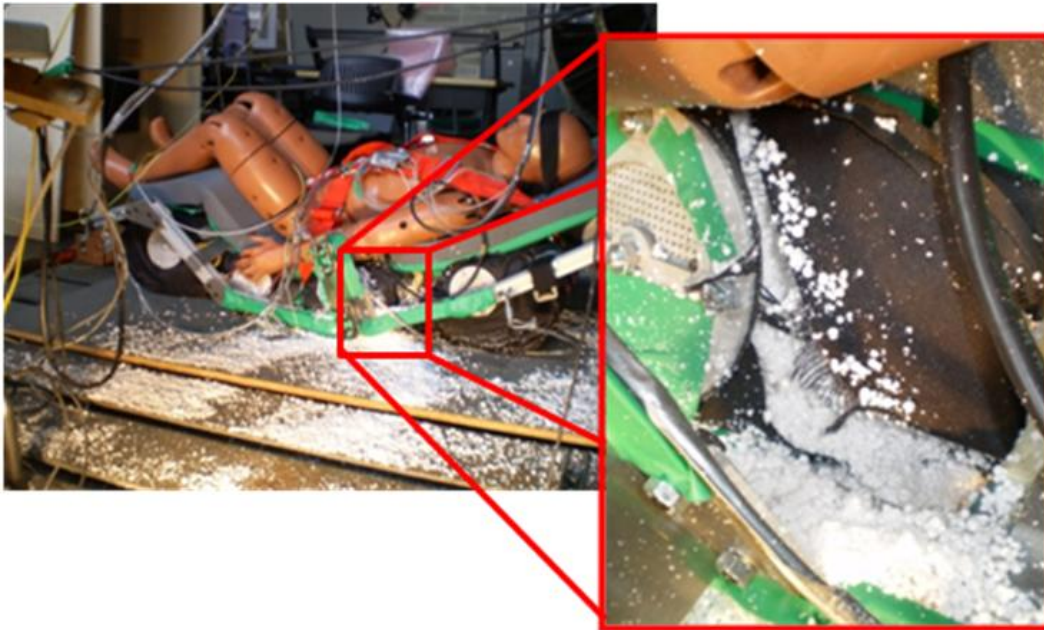
Figure 4-13: Test Failure from a 5 foot Drop Height
