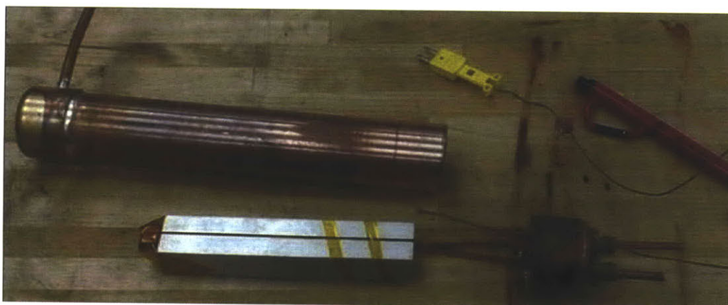
Figure D.7 Prototype copper pipe with HTS wires inside aluminum block
