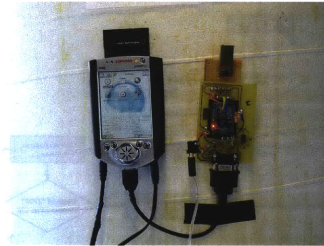
Figure 4-3 Sound Collecting Module (SCM): From left to right: PDA connected to TB
