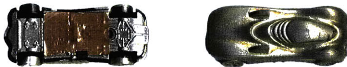
FIGURE 3.3.7 A TouchTag enabled toy car with an RFID tag chip. It could still function if coated with a nonconducting outer surface.
