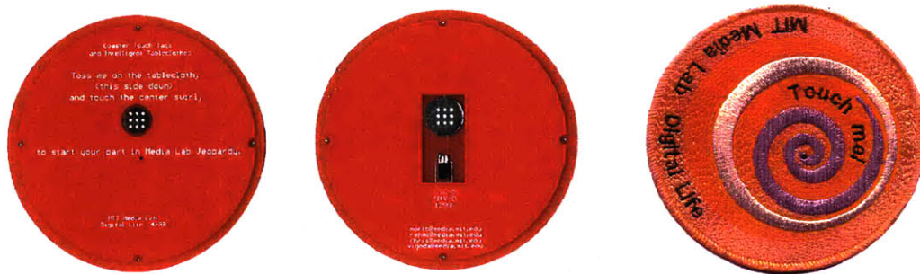
FIGURE 3.3.6 TouchTags used as tabletop login tokens for “Tablecloth Jeopardy Game” TTT Spring 1999. Views from left to right: Bottom, Top (with Swatch RFID tag chip), and “Ebroiderey [POS97]” Top Cover.
