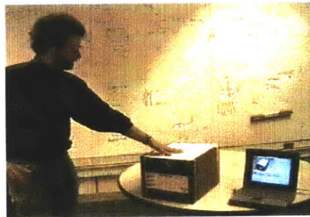
FIGURE 3.3.5 Retrieving information about a package by touching it. The box contains an electrostatically coupled RFID tag. Professor Gershenfeld is wearing a TouchTag reader in his shoe which reads the tag and outputs this information to the laptop. The laptop displays information about the box.
