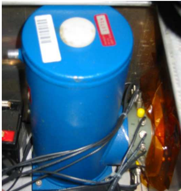
Figure 3-5: DIII-D PCI detector is contained in a LN 2 dewar
