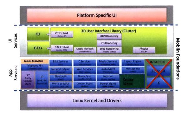
Figure 20: PSG Platform stack evolved from Moblin (Adapted from Moblin.org)
