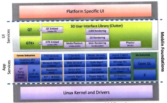
Figure 19: Intel's Moblin Software Stack (source: www.Moblin.org)
