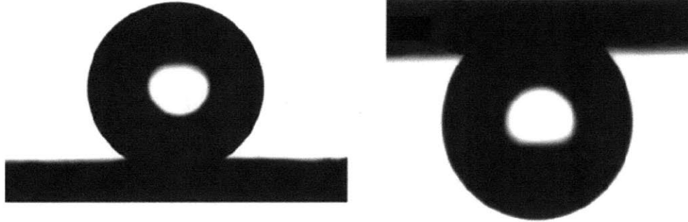
Figure 2.4.3 Adapted from Feng et.al., the droplet on the left shows a water droplet adhered to a sample of rose petal. From this image, it is clear that the contact angle is within the superhydrophobic range of >150 degrees. The droplet on the right is a water droplet on the same sample of rose petal now inverted to show that the droplet does not roll off the rose petal even when upside-down (4115).
