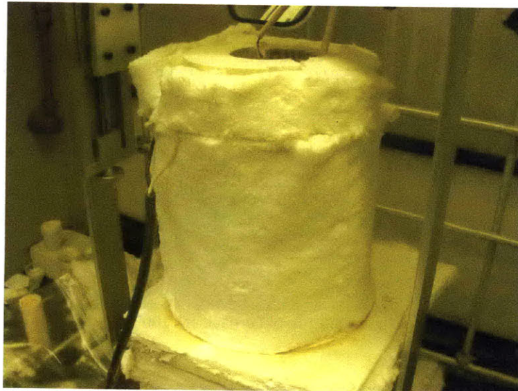
Figure 3.11 Furnace After Partial Replacement of the Heating Elements
