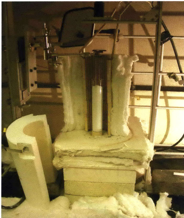
Figure 4.3.1 Furnace and Salt Sample Before the Test
