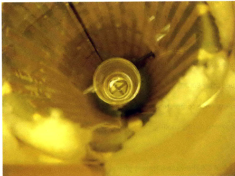
Figure 4.1.5 Salt Completely Melted and Transparent
