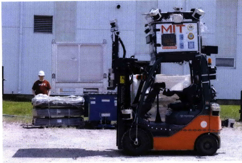
Figure 1-2: Image of the autonomous forklift of Agile Robotics Lab at MIT [4]. Photo courtesy of Jason Dorfman.
