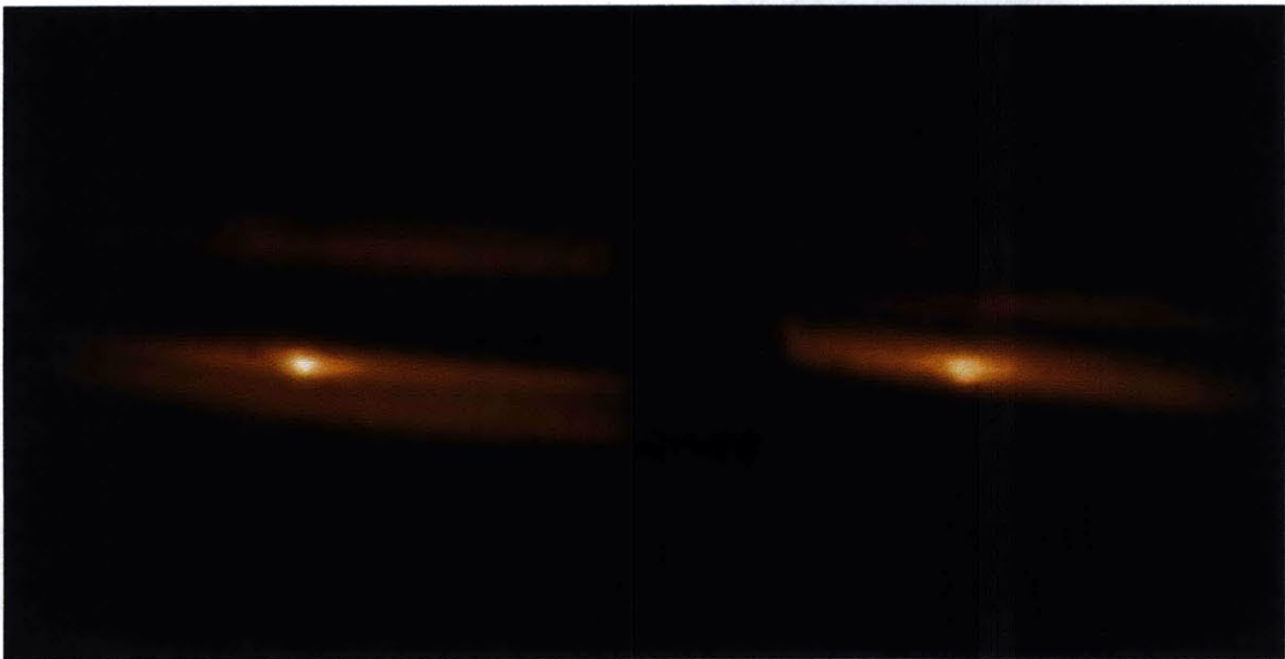
Figure 4-9: Image from shot 1080501011. Image has been processed to bring out its features, in particular what we are seeing is logarithm of the intensity recorded by the CCD above some threshold background value. The display is normalized such that the highest numerical value is represented as white (255) and the lowest as black (0).
