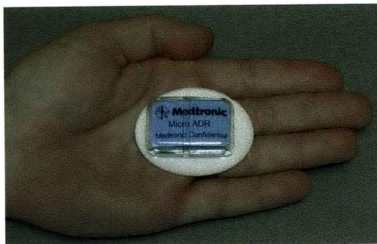
Figure 2-6: The Micro Ambulatory Data Recorder ( $\mu$ ADR) is a small device approximately 1.5 x 2 inches which is adhered to a subject's gluteal region. It encases a triaxial accelerometer (ADXL-330, Analog Devices) as well as a data recording device.
