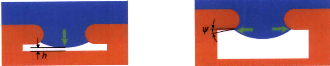
Figure 4.8 Schematic overview of two failure mechanisms and criteria - the texture angle ( \psi ) and height of the lowest point of liquid ( h ).
