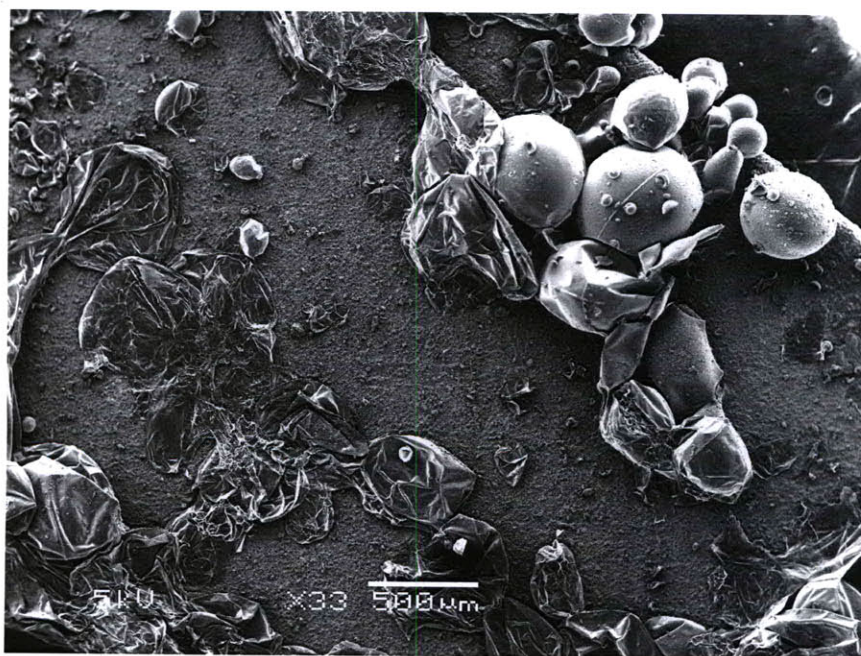
Figure 4-3: Polymeric bubbles formed on the underside of a horizontally positioned filter paper substrate.
