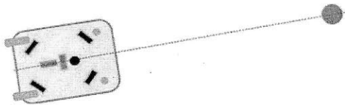
IV - 1: Point to point control: robot first aligns with desired endpoint, then drives in a straight line
