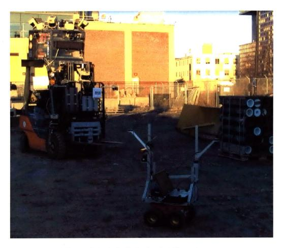
Figure 5-1: Agile Robotics forklift and rover
