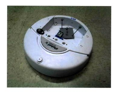
Figure 4-11: iRobot Create with xBee-PRO wireless serial module connected order to send actuation commands.
