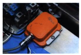
(b) Xsens MTi IMU —  $0.05^{\circ}$  angular resolution
