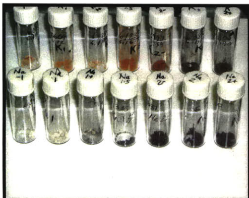
Figure 6: Isolated sodium and potassium mono- and diselenides. Potassium selenides are seen in the back row of vials, and sodium selenides are seen in the front row. From left to right there is an increasing Se:M ratio: 0.95, 1.0, 1.05, 1.5, 1.95, 2.0, and 2.05.
