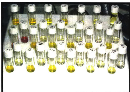
Figure 8: CdSe nanocluster solutions after ripening. The pale yellow solutions were ripened in pyridine, the yellow solutions were ripened in methanol, and the red solutions were not ripened and the synthesis was carried out in the absence of pyridine.
