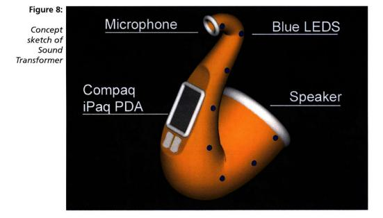
When the user sings into the device, the audio is wirelessly transmitted to a remote server. The audio content is then analyzed for pitch, volume, brightness, and spectrum. The analytical results are then fed into a software synthesizer to create an audio stream. This transformed audio is then returned to the device, amplified, and played out loud.
