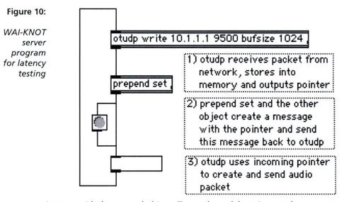
interact with the network driver. To test these delays, I created two more programs, one for the iPaq and the other for the MAC server. The iPaq program sends input from the microphone to the server. It simultaneously checks for audio packets from the server. This program directs all incoming audio packets to the speaker.
