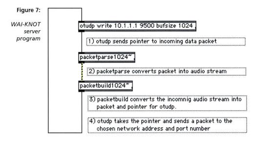
the incoming MAX/MSP audio stream and passes a pointer to otudp. Otudp uses this pointer to create a packet and then sends packet to the chosen network address and port. See figure 7.
