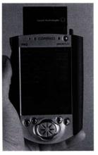
Currently the smallest computer capable of running an 802.11b network card is a Compaq iPaq. The iPag has a 200MHz arm processor with sound card capable of full duplex 44.1KHz 16bit audio. Though the iPaq comes with Windows CE installed, I discovered that Windows CE doesn't support full duplex audio. Therefore, I installed Linux on the iPaq. More information on running Linux on a Pocket PC can be found at www.handhelds.org.
