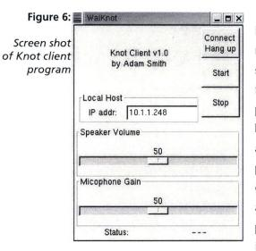
Next, I created a graphical user interface which allows the user to connect to a remote computer over a UDP socket using 1024 byte packets. See figure 6. After connecting, the user then presses the start button. Once the start button is pressed, my program records audio packets from the internal microphone and sends them to the remote computer. The program also listens for audio packets from the remote computer. When receiving an audio packet, it sends the audio data to the sound card
