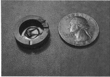
Figure 3-10: A Zowie tag, with a US quarter shown for scale.
