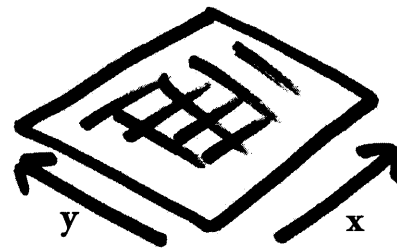
Figure 3-24: In turn the board underneath the tags strobes every antenna line along the X axis, and then every line along the Y axis.
