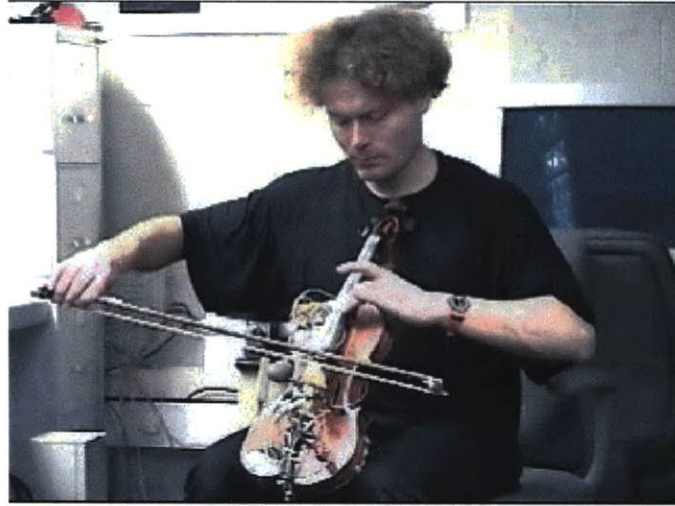
Figure 10-5: A one string digital violin (fall 1998). The strings are muted. The instrument functions as a sensor input device for the single-string model, ranging over two octaves. A sound clip is available from [WEB].
