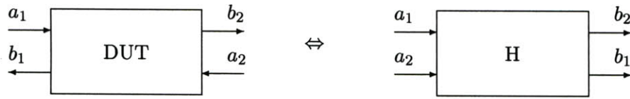
Figure 7-3: Device under test (DUT) characterized by its transfer function.
