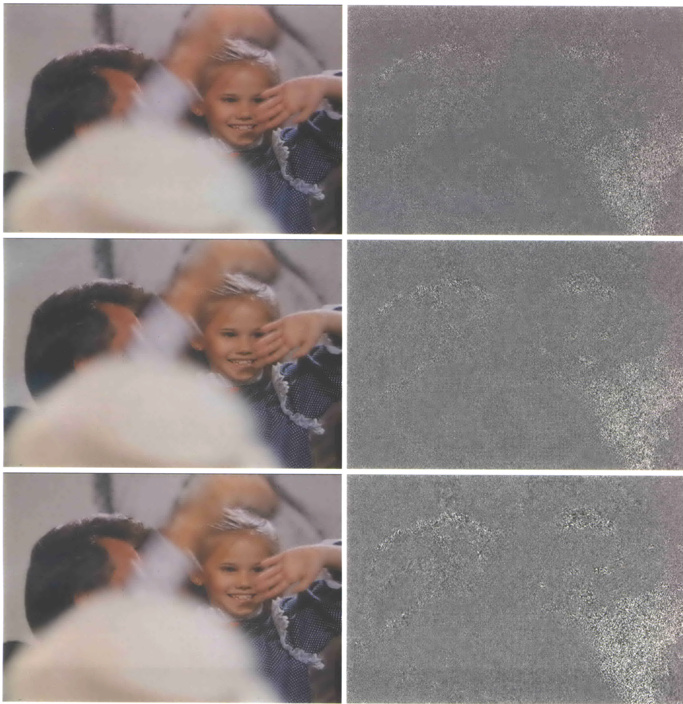
Figure 5.2: MPEG-2 with high-rate quantization. Left: reconstructed images. Right: coding errors magnified by 10. Top: at 20 Mbit/s, center: at 15 Mbit/s, bottom: at 10 Mbit/s.
