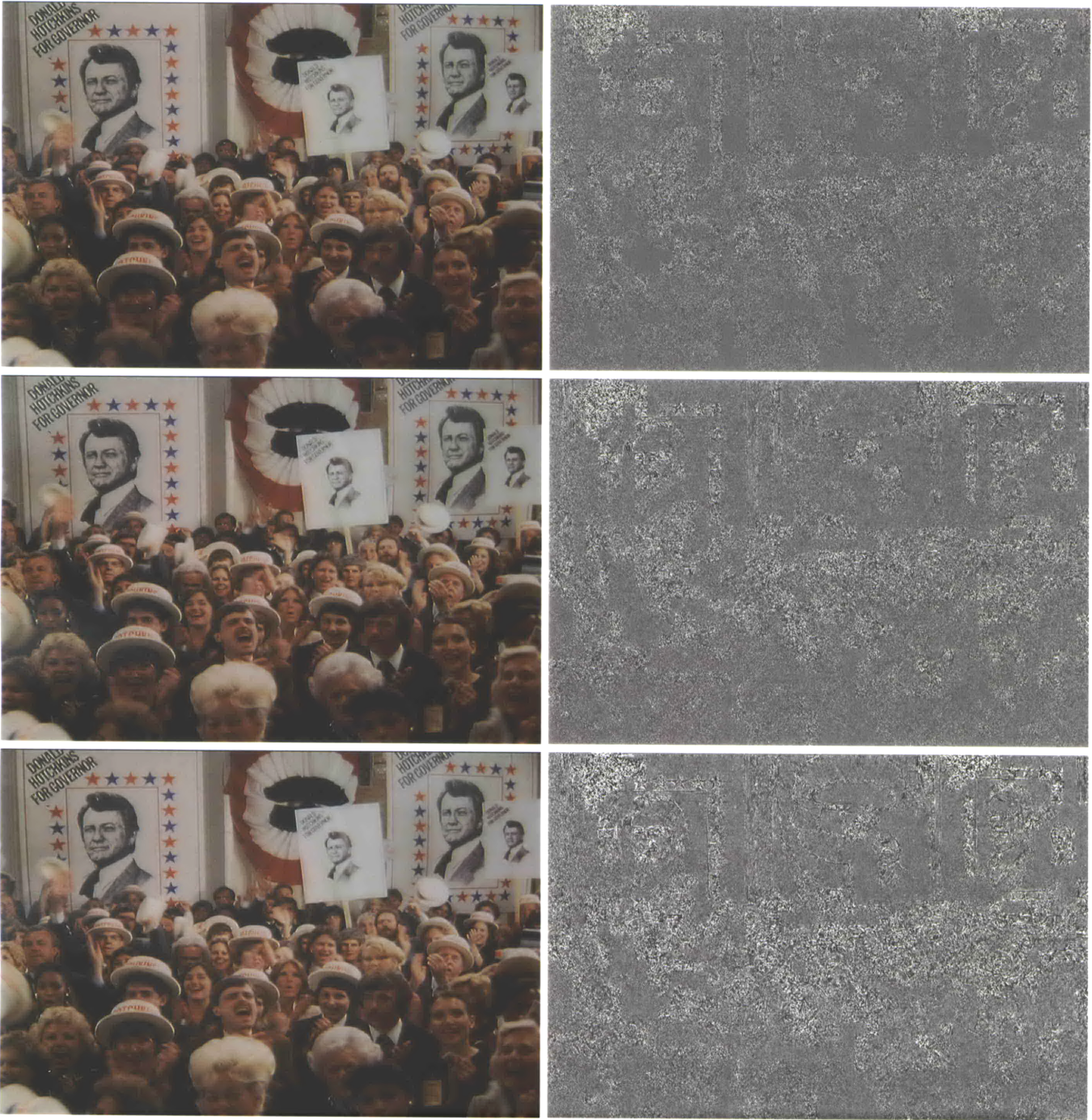
Figure 5.3: MPEG-2 with high-rate quantization. Left: reconstructed images. Right: coding errors magnified by 10. Top: at 20 Mbit/s, center: at 15 Mbit/s, bottom: at 10 Mbit/s.
