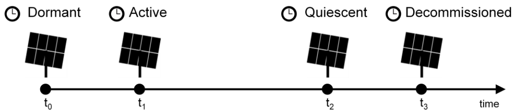
Figure 11: Element reconfiguration sequence. An element may experience several operational states throughout a campaign including dormant before delivery, active or quiescent during operation, and decommissioned state to signal availability of parts for scavenging.
