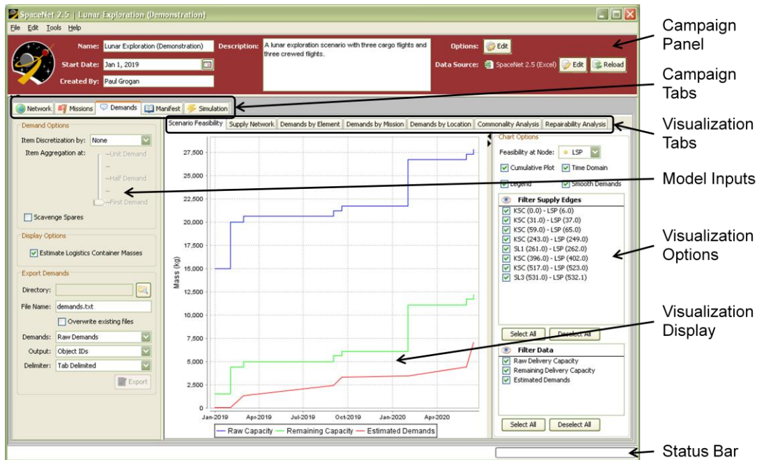
Figure 31: SpaceNet 2.5 user interface. The SpaceNet GUI guides users through the process of modeling and analyzing exploration campaigns.
