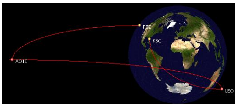
Figure 50: NEO sortie network. Visualization of space edges between launch, low-Earth orbit, the near-Earth object 1999 AO10, and splashdown in the Pacific Ocean.
