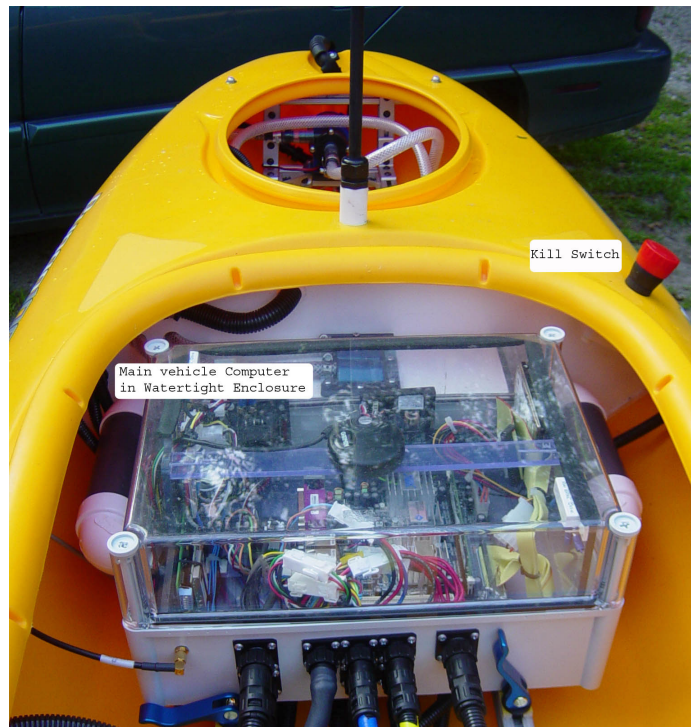
Figure 6-2: Main on board computer and 802.11b (Wi-Fi) radio [9].
