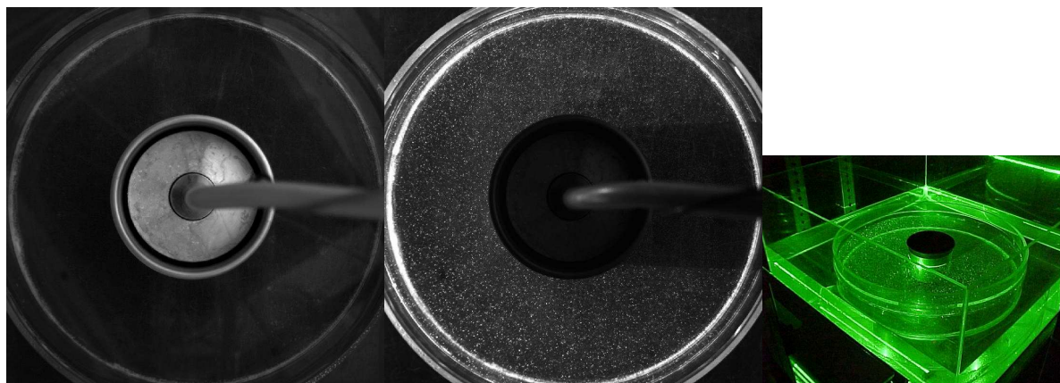
Figure 4. The camera's view of the rotating annulus in visible light is shown on the left. The corresponding view in laser light depicts the embedded particles and is shown in the middle image. A picture of the laser illuminating the tank is shown on the right. Notice the shadow due to the chiller in the middle. The square tank is used to prevent the laser light from bending at the annulus interface.
