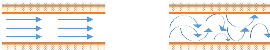
Figure 1.8 A representation of laminar flow with separate flow layers (left) and a turbulent flow with crossed-mixed flow layers (right).
