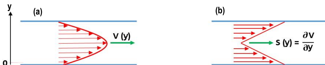
Figure 1.9 (a) Side view of velocity profile and (b) shear rate distribution in a simple geometry with laminar flow.
