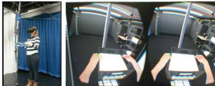
Figure 2 : Use of the haptic interface and head-mounted display (Left). Virtual rendering of this handling through the head-mounted display (Right).
