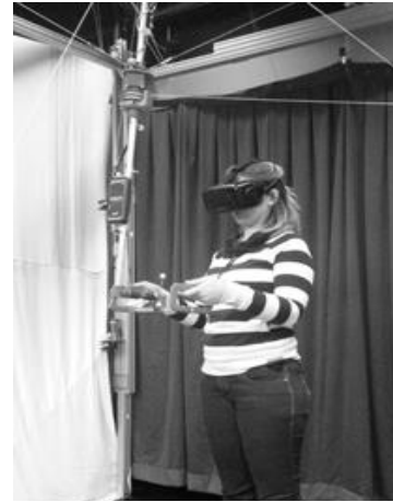
Figure II-3 : Use of the cable-driven robot and head mounted display
