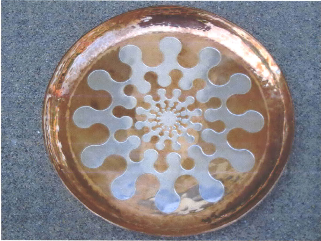
Figure 60 Copper craft etched and plated with a pattern created with Estampa
