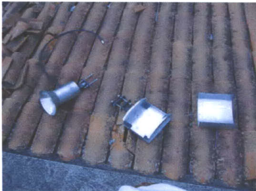
Figure 14 Wave-guide antenna and weather proof casing manufactured in the CECATI
