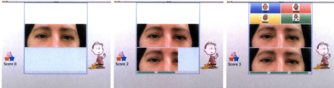
Figure 4-2: When a new puzzle is first presented only the target puzzle is shown (left). During construction the physical pieces placed on the board appear in the corresponding location in the digital interface (center). When correctly constructed the expression choices are presented with text and picture icons for choosing the expression label (right).
